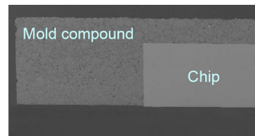
Fig. 11 molded die in a RCP package
